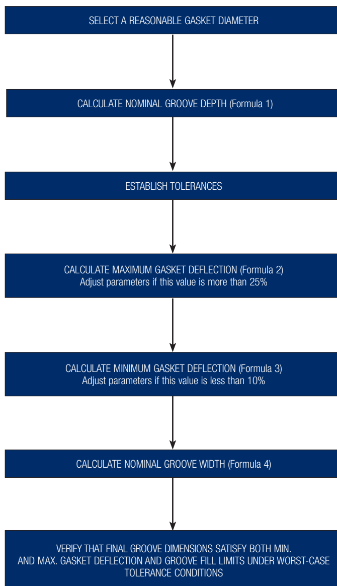
Figure 3-23. Procedure for Calculating Solid O Gasket and Groove Dimensions
